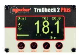
TruCheck™ 2 Plus display showing below target tolerance
