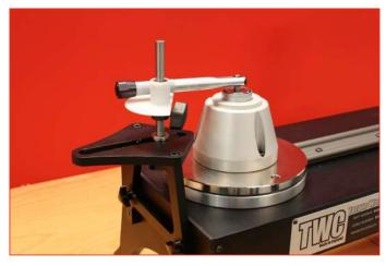
60318 Static Transducer Support Kit and 60319 Short Length Reaction Post
