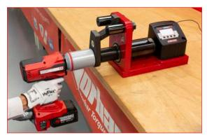
TruCheck™ 2 Plus 1100 shown with a Power Tool Test Fixture (not included - see page 27) allowing for cost-effective checking of power tools
