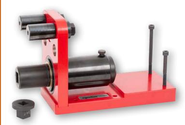
The Power Tool Test Fixture for TruCheck™ 2 is a simple, robust device that allows non-impacting power tools up to 2,100 N·m to be tested. A system comprises the Test Fixture with a TruCheck™ 2 Plus (to be ordered separately), either the 1,100 N·m or 2,100 N·m models, depending on the torque capacity required. The universal torque reaction arrangement will suit reaction arms supplied as standard with most Norbar and other pneumatic, electric and cordless torque tools.
