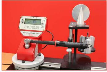
60323 Pro-Test and Static Torque Block Adaptor Kit
