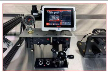
T-Box™ 2 at the centre of a test bench for hydraulic torque wrenches
