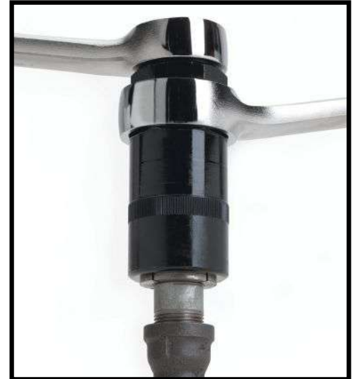
The Tight-Grip Nipple Tool in use. One wrench holds the housing in place while the other wrench turns the top nut, clamping the collet and housing assembly onto the nipple. The housing, collet, and nipple then turn as one.
