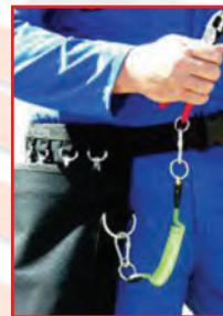
9. Select a lanyard to suit the weight of tool you intend to use. The weight of each tool can be found on the kit data sheet while each lanyard is fitted with a safety label stating the maximum tool weight it is rated for.
