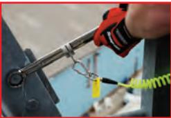
4. A Snap-Coil is not designed to "breakaway" from the operator if a tool is snatched into moving machinery. No "breakaway" device can be guaranteed 100% effective so best practice is for machinery to be shut down, isolated and a safe working area designated before any work is undertaken nearby.
