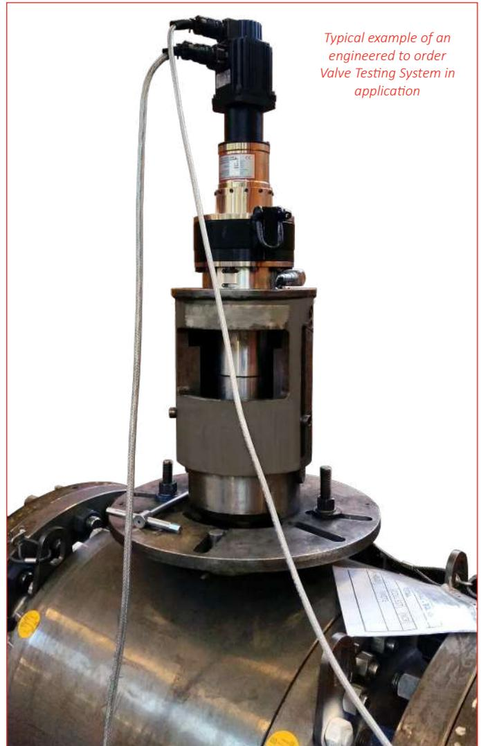
*Typical example of an engineered to order Valve Testing System in application*
