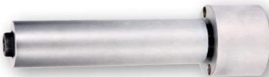
The Norbar Joint Simulation Rundown Assemblies are designed to simulate the working conditions of screwed or bolted joints. Used in conjunction with a Norbar transducer and display instrument, the output of torque controlled power tools can be measured against a range of simulated joint rates, from hard through to soft.
