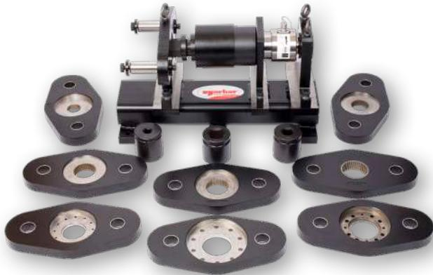
Power Tool Test Rig
