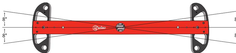
Additionally, the beams are designed to apply load on a vertical plane which cuts through the square drive inside the transducer. This minimises bending moments on the transducer and for safe operation, ensures that the beam will not fall out of the transducer.
