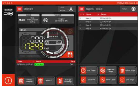
Displaying transducer reading alongside target selection
