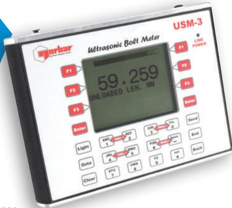
Ultrasonic measurement provides a very precise method of determining the elongation of a fastener due to tightening. This elongation is proportional to the load force generated by the fastener.
