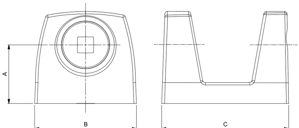
Bench stands ensure the correct mounting of Norbar's Static Torque Transducers up to 7,000 N·m (5,000 lbf·ft).
