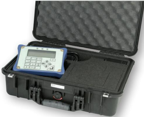
TTL-HE is a portable torque measuring instrument designed for use in harsh environments. The TTL-HE operating on battery power with one of the 'HE' range of transducers connected, has an ingress protection rating of IP65/IP67. Typical operating environments are where high humidity, water or salt water spray and dust may be an issue. Features include; 10 measurement modes, 13 units of torque (with additional user units feature), 12 pairs of limits and text displayed in 11 languages.
