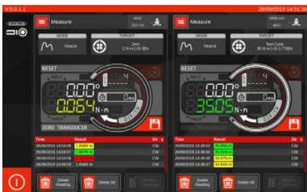
Displaying 2 transducer readings simultaneously
