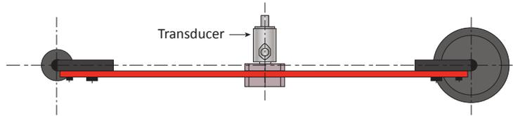
Torque is generated by the application of a known force at a known radius from the centre of rotation of the torque transducer.
